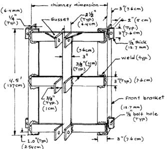
fig. 3. Construction details of front bracket assembly.
